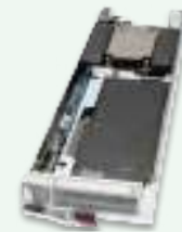
SBA-4119SG GPU Model with 2 GPUs, M.2 NVMe
