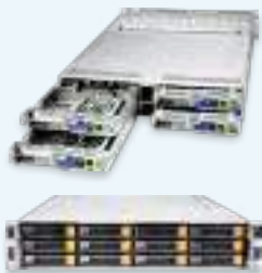
SYS-621BT-H Series 3x 3.5" NVMe/SAS/SATA drives (per node)
