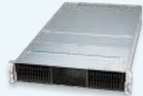
SAG-221E-NE324R Up to 24 EDSFF (E3 7.5mm NVMe SSD)
